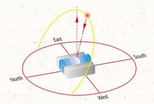
**Summer** - When the path of the sun is high, RFX reflects away the sun's rays, preventing heat from penetrating into the structure
