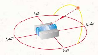
**Winter** - When the path of the sun is low, RFX allows penetration of solar energy through the panel, providing a natural heating source.
